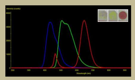
The entire 400 nm to 700 nm visible region is covered by the three LEDs (the small peak in red colour is a weak secondary emission from Spectrafill red LEDs). White light synthesised by combining the light from three separate Spectrafill devices has a significantly flat spectral distribution – ideal for
